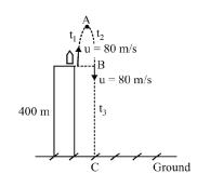
Velocity of the bullet at point A,  $V_A = 0 \text{ m/s.}$  a = -10 m/s V = u + at  $0 = 80 - 10 t_1$   $t_1 = 8s$   $t_2 = t_1$  (as there is no air resistance) Calculation for  $t_3$ Velocity of the bullet at point B,  $V_B = u = 80 \text{ m/s}$ h = 400 m
